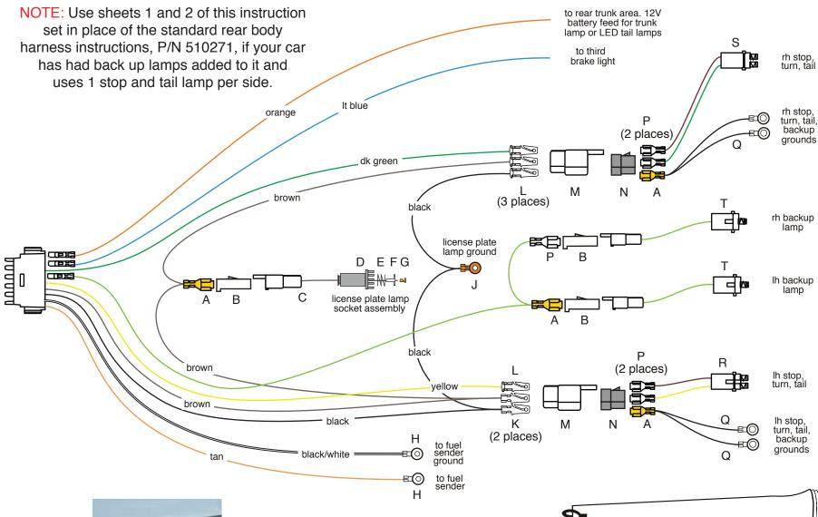
1961 - 1962 Corvette with Back Up Lamps and single Stop/Tail Lamps (2 lamps per side)
